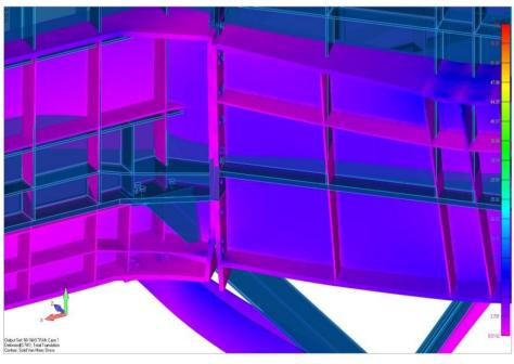
Regarding enormous loading from coal ash (9860 kN), the connection between beam and column is very important. It can be clearly from next picture.
