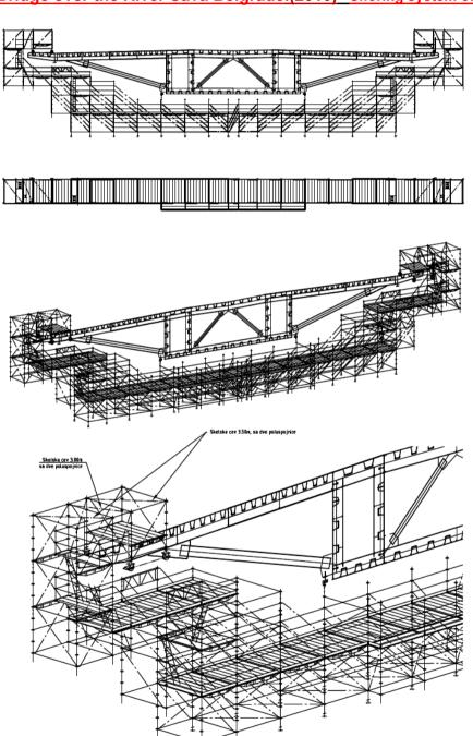
Modeling and analysing of structure (FEM/FEA) was done with software software package, **FEMAP**, and calculation using software **SAAD PRO**.
