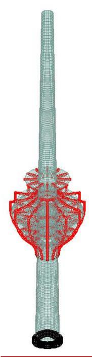
Mesh of the Finite Elements Model for static, dynamic and stress analysis.
