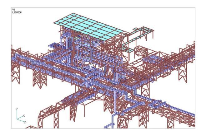
Modeling and Analysis for the pipe racks for the Energy Plants in Turkey (2001). Joining the modeling for the piping and for the racks was done using the translator we have created for the specific purpose.
