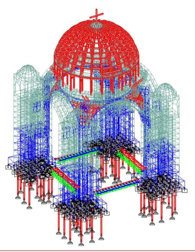
Mesh of the Finite Elements Model for static, dynamic and stress analysis.
