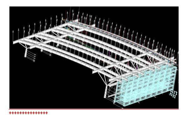
Static analysis of tunnel shell -Metrostation KAZAHSTAN II (May 2008)
