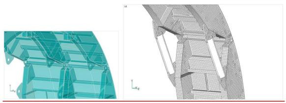
Mesh of finite elements with the materialization of the cross. sectional members. +++++++
